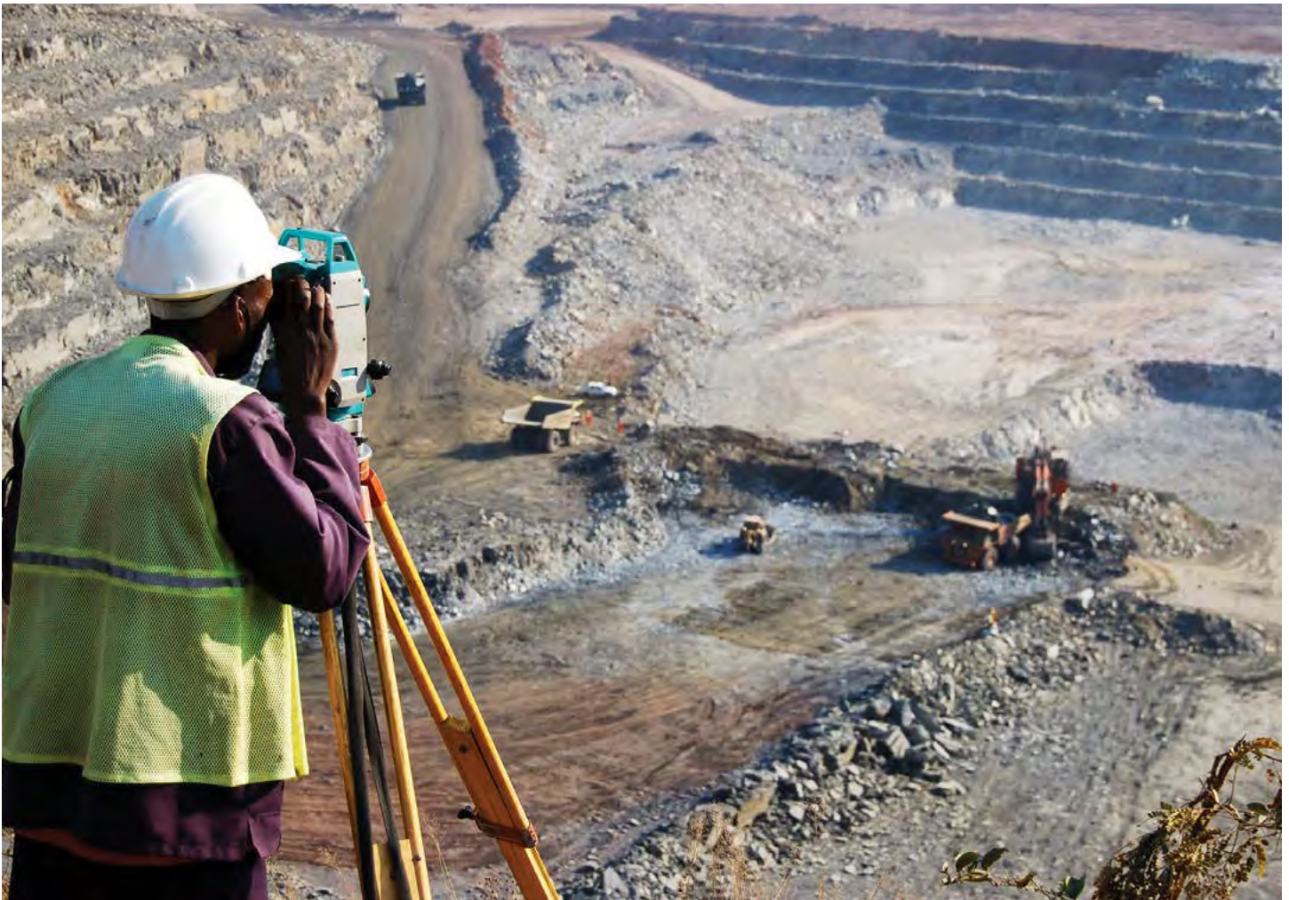
A locally employed surveyor at an open-pit copper mine in Zambia peers through a theodolite to record the daily changes in the mine and to help guide mining activities. (Photo by mabus13/iStock)
